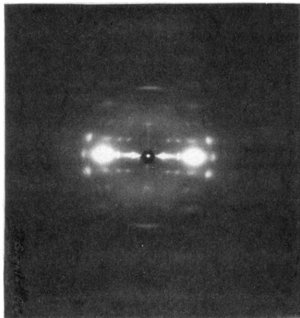
Figure 1. Wide-angle X-ray diffraction photograph of the TPA/PHQ/PEHQ copolyester fibers annealed at 590 K for 4 h under load (medium exposure time).
